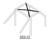
Drawing of the roof reinforcement
