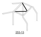
Drawing of the roof reinforcement
