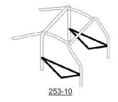
Drawing of the doors reinforcement
