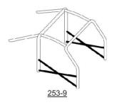
Drawing of the doors reinforcement
